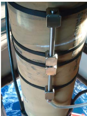
INTEGRISTICK™ strapped to a riser
