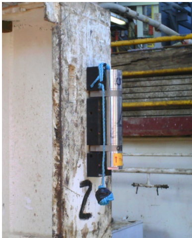
Data logger installed on BOP frame
