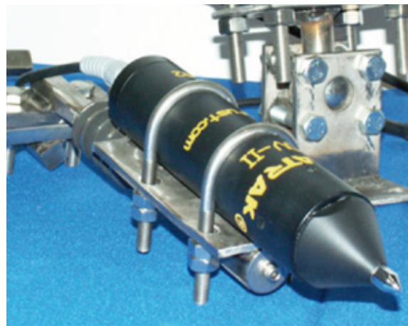
ROV-II The ROV II Probe shown on the compliant T-Handle mount
