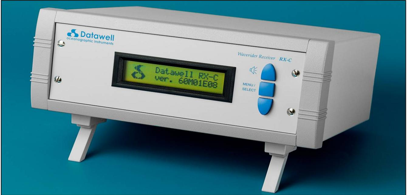
The RX-C is a dedicated HF link receiver that supports all Datawell Waverider buoys fitted with the standard HF transmitter. The RX-C supports both the "HXV" format and the "HVA" transmission formats. The HXV format is used by the current buoys. The HVA format is used by the DWR4/ACM buoy.
