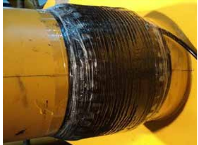
Photo 2: Strain gauge assembly ready for deployment protected by Pulse proprietary water sealing package
