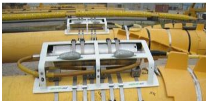
INTEGRISTICK™ and INTEGRIPOD™ deployed on a steel catenary riser with protective cage
